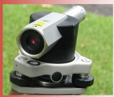
Safe output as a Class 2M laser device makes it safe to use under all mining, building and construction applications, including underground coal mining. The BLX-635S is the bench-mark laser alignment tool in 2013 and beyond for alignment and laser safety barriers in mining automation applications.
