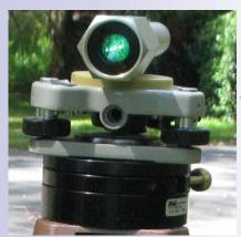
BLX-515S shown on tripod-mounted rotational adjustment base with tribrach for precise vertical tilt and fine rotational adjustment. Laser is removable from the tribrach for battery change. V-R adjust.
