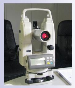
BLX-635S shown mounted in functional electronic theodolite for use in non-hazardous areas where non-Intrinsically Safe devices are permitted. An identical version with the electronics removed for use in hazardous areas is available for simple and precise use of the theodolite mechanical adjustments. Precise H-V-R adjustments.
