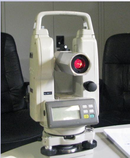
BLX-635S shown mounted in functional electronic theodolite for use in non-hazardous areas where non-Intrinsically Safe devices are permitted. An identical version with the electronics removed for use in hazardous areas is available for simple and precise use of the theodolite mechanical adjustments. Precise H- V-R adjustments.
