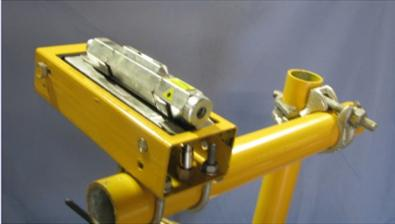
BLX-515S shown mounted in precise H-V mount for mounting to horizontal hangers in underground coal mines. The laser is removable from the mount to easily change batteries.
